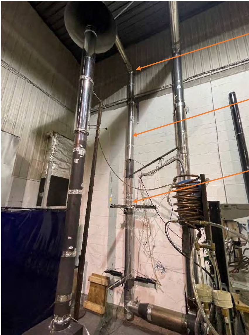
Total length between hood and sampling port : 22 feet.
