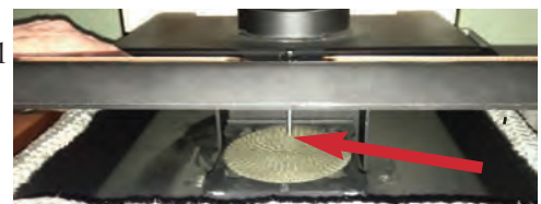
When the lid is closed, the end of the probe is less than 1 inch away from the catalyst (see above)
